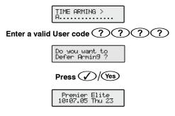
The system will return to Time/Date displayed on the keypad and defer Time Arming of the system, for example by 30 mins, or whatever has been programmed as the defer arming time.
