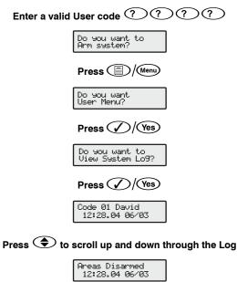
Press (Area) to toggle between the area information and the time/date Press (Area)/(Part) to display zone text (where applicable)
